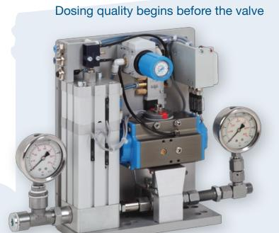
The patented DAS 120/12 Pressure Balance System limits the high pressure within supply systems for industrial greases and highly viscous fluids before they are fed into the dosing components, and prevents pressure fluctuations.
