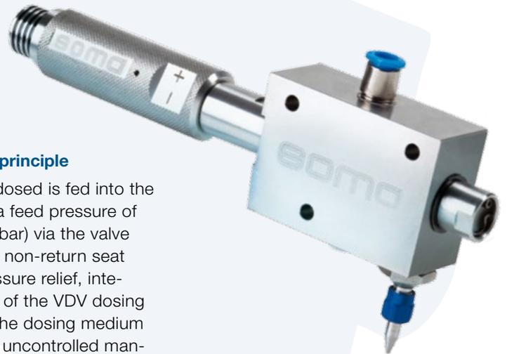
The SOMA volumetric dosing valve (VDV) was developed for use in dosing processes where the reproducible and contact dosing of precise volumes is of great importance regardless of fluctuations in primary pressure and the viscosity of the lubricant being dosed.
